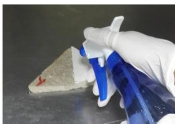
Figure 3: Procedure A: Sample sprayed with microorganisms
